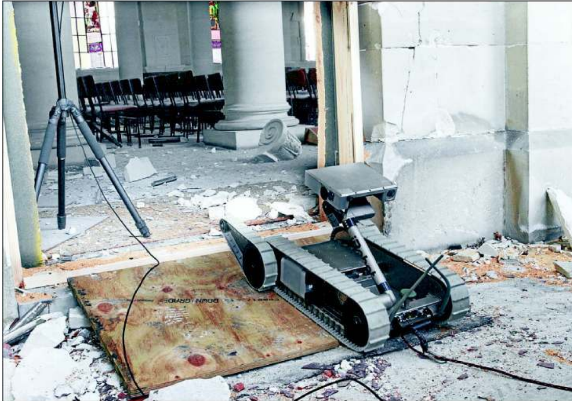
Assessing the damage: An army robot makes its way into the Cathedral of the Blessed Sacrament.
